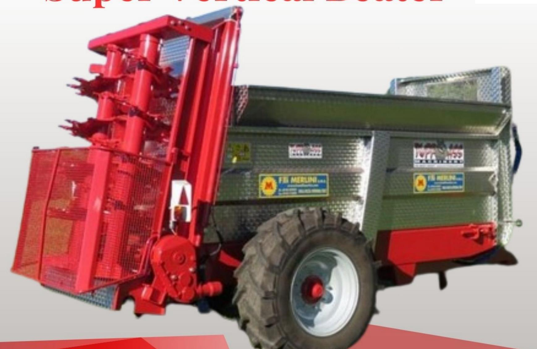
The heavy duty floor chains feed into the heavy duty 10mm roller beaters featuring bottom spreading plates. These plates ensure better spreading of fine materials like chicken litter, lime and gypsum.
